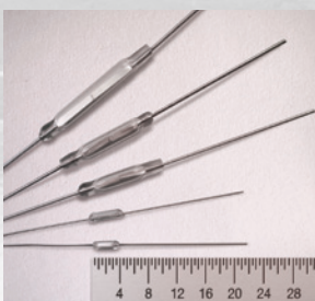
Magnetic reed switches for position sensing
