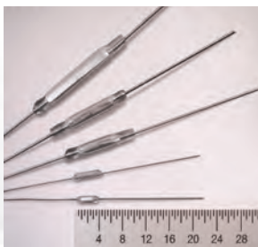
Magnetic reed switches for position sensing
